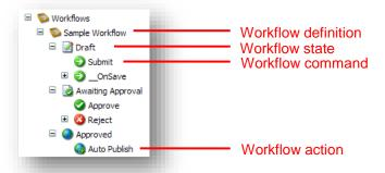
Workflow commands move items from one workflow state to another. Every workflow command has a corresponding definition item. The definition items for commands are stored under the corresponding workflow state definition item. The workflow command is only shown when the selected content item is in the corresponding workflow state.
